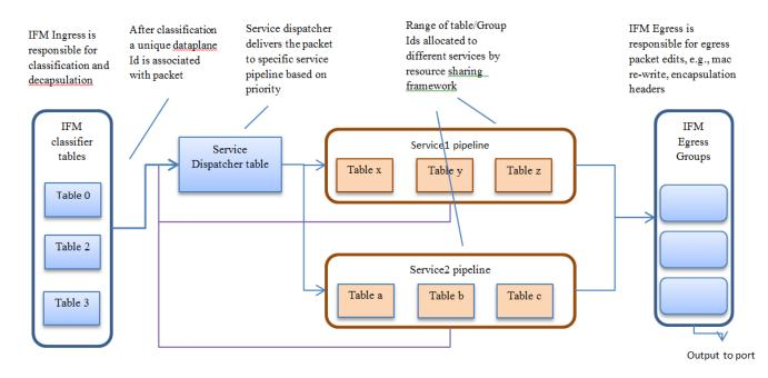
On different application request, Interface Manager returns the egress actions for interfaces. Service modules program use these actions to send the packet to particular interface. Generally, these egress actions include sending packet out to port or appropriate interface egress group. With the inclusion of the egress dispatcher table the egress actions for the services would be to
